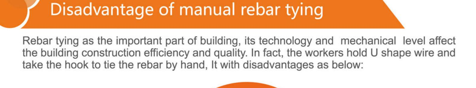
Heavy works Low efficiency Knots tightness are nonstandard Pressed schedule 6. Wrist joints hurt easily Wire waste
